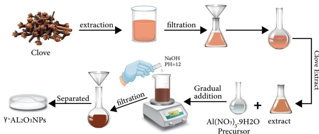
Figure 2. The preparation steps of \gamma - Al 2 O 3 NP powder using clove extract and aluminum nitrate. Nona hydrate in alkaline media.
