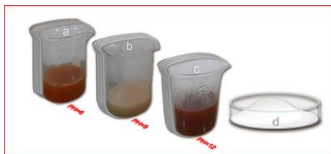
Figure 3. Color change of solutions in the alkaline media with \text{Al}(\text{NO}_3)_3 \cdot 9\text{H}_2\text{O} and, bio-reductors of clove extract (a) brown, (b) Peggy, (c) dark brown, and (d) the final product of \gamma - \text{Al}_2\text{O}_3 NPs powder.
