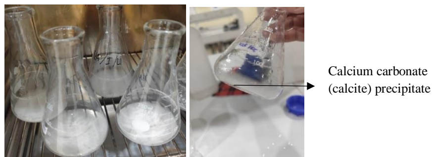
Figure 4. Calcium carbonate precipitation test using NB-U/Ca medium at 30^\circ\text{C} at 130 rpm speed for 7 days
