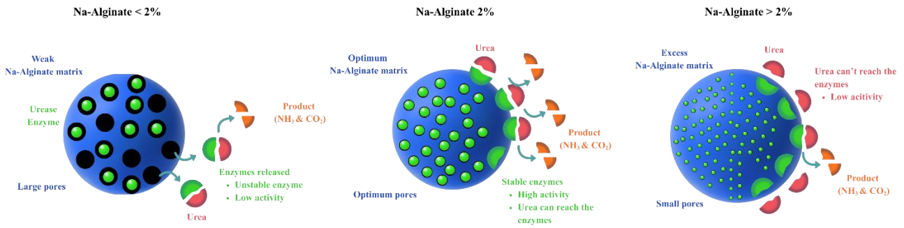
Figure 3. Illustration of the effect of Na-alginate concentration on immobilized enzyme activity
