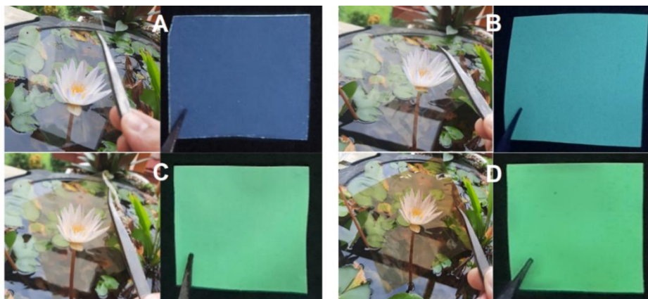
Figure 1. Photographs of gelatin/C-dots composite films with various C-dots content a) 0%; b) 0.1%; c) 0.5%; d) 1% under daylight (left) and UV lamp (265 nm, right)
