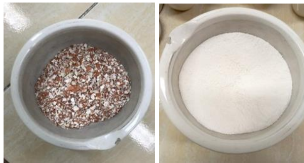
Figure 1. Egg shell A) before and B) after the calcination process
