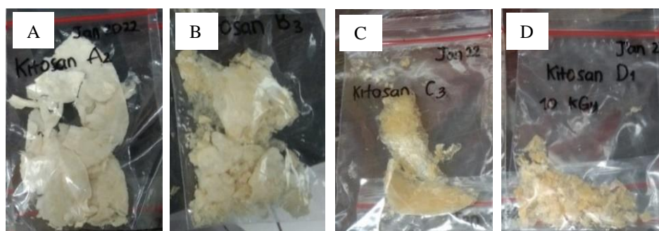
Figure 3. Discoloration of chitosan A (5 kGy, 5 mL), B (5 kGy, 10 mL), C (10 kGy, 5 mL), and D (10 kGy, 10 mL)
