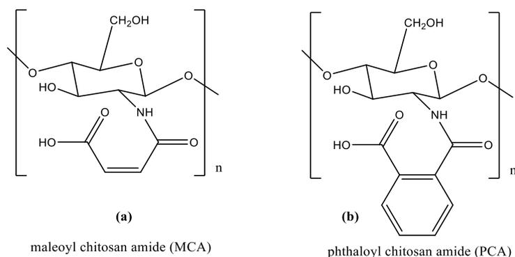
**Figure 3.** Maleoyl chitosan amide (a) and Phthaloyl chitosan amide (b)
