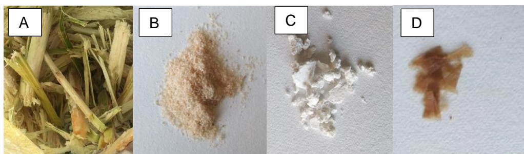
Figure 1. a) Sugarcane bagasse (SB); b) SB After alkali treatment; c) Cellulose; d) Nanocellulose.
