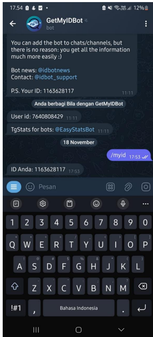
Figure 5. Procedure for retrieving the Telegram chat ID using the Telegram API
