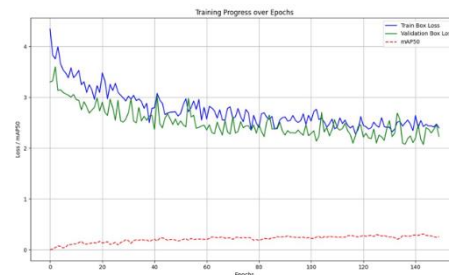
Figure 7. Training, validation, and mAP50 result for tight dataset - YOLOv8n.pt
