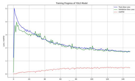
Figure 5. Training, validation, and mAP50 result for loose dataset- YOLOv8 Original
