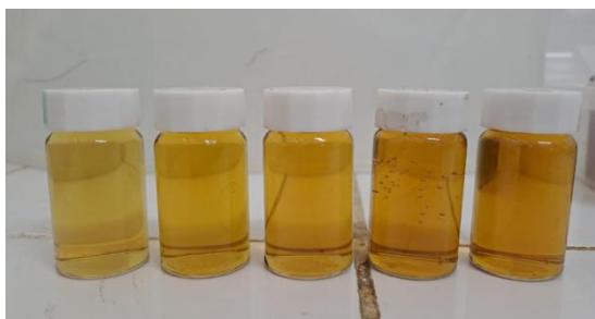
Figure 2. Colloidal silver nanoparticles mediated by P. buxifolius leaf extract (extract concentration variations from left to right 0.01, 0.02, 0.03, 0.04, and 0.05%)
