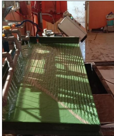
Gambar 1. Percobaan Shaking Table
