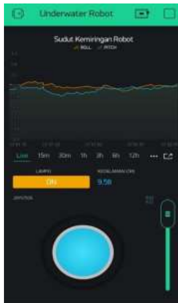
Figure. 8 Overall Control System View on Blynk
