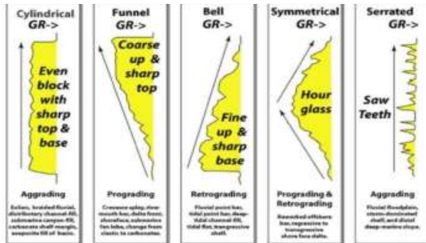
Figure 2.1 Response of gamma-ray log to variations in grain size and depositional environment [9]
