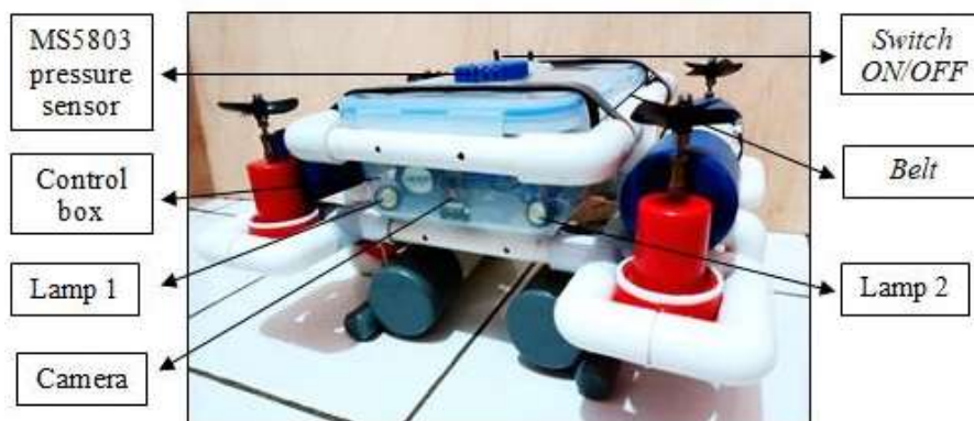
Figure. 3 Underwater Robot Design Result
