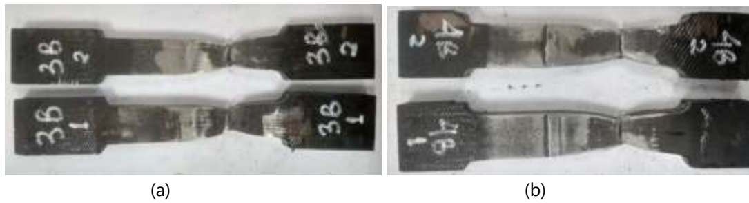
Figure 2. (a) Fracture specimens for three layers weldment, (b) Fracture specimens for four layers weldment
