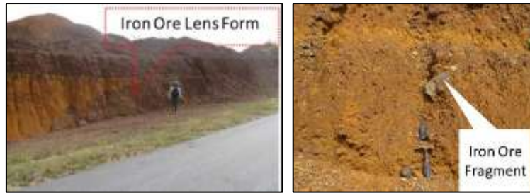
Figure. 2 Iron Ore Fragments in Soil Layer on Any Places Forming the Lens [5].
