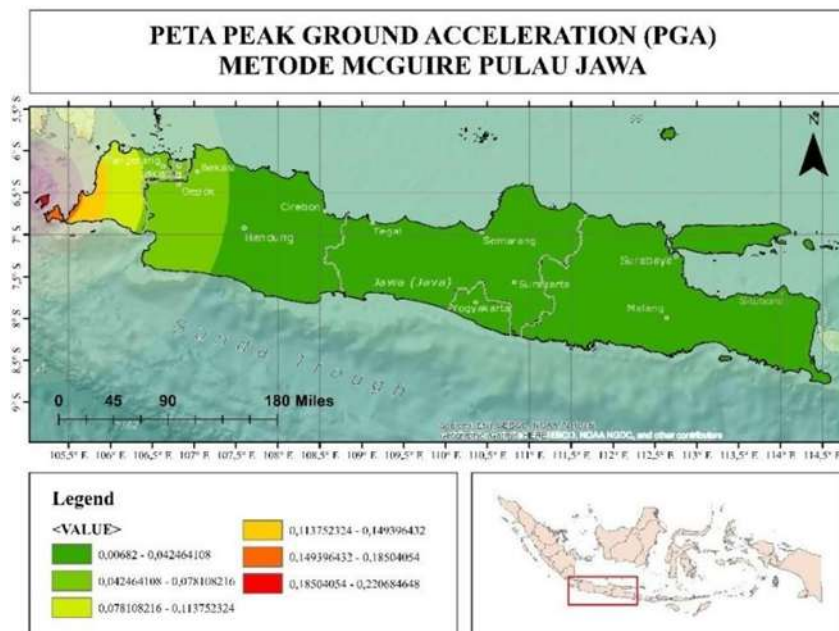
Figure 4. Peak Ground Acceleration (PGA) Map of Java using McGuire’s model Figure 4 illustrates the spatial pattern of Peak Ground Acceleration (PGA) across Java Island derived from the McGuire attenuation model. The resulting distribution demonstrates considerable variability in PGA values, ranging from 0.00682 g to 0.2206 g throughout the study area. The highest PGA values are concentrated in western Java, particularly within the Banten region, where estimated accelerations range between 0.1493 g and 0.2206 g. These areas are represented by orange to red color gradients on the contour map, indicating the strongest levels of expected ground shaking. The elevated PGA values observed in this region are consistent with its tectonic setting, which is strongly influenced by the Sunda subduction zone and the activity of major fault systems such as the Cimandiri Fault. Consequently, western Java exhibits the highest level of seismic hazard among the regions analyzed. In contrast, the majority of Central Java, the Special Region of Yogyakarta, and East Java are characterized by lower PGA values, generally below 0.0781 g, as indicated by the predominance of green shades on the map. These lower values suggest a
