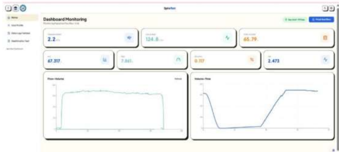
Figure 6. Real-time display of respiratory parameter data on the IoT Dashboard interface
