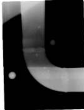
Figure 7. Insulated Pipe Using 180kV, 3mA, and 40 Second Computed Radiography
