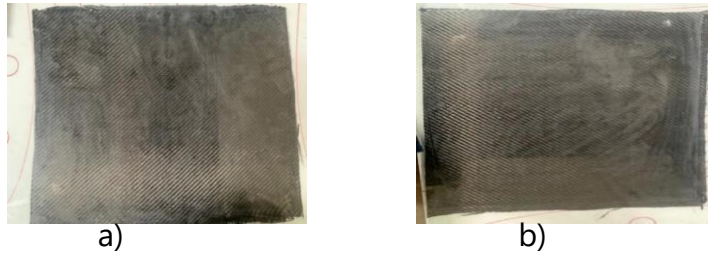
Figure 3. The Results a) The Vacuum Infusion b) Vacuum Bagging Processes
