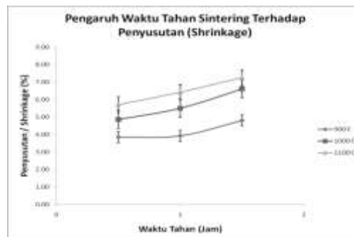
Figure 8. Graph of Relationship between Sintering Resistant Time and Shrinkage of Mo/Al 2 O 3 Composites.
