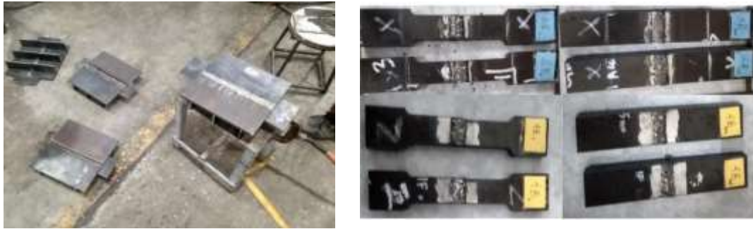
Figure 1. (a) Welding jigs for each plates, (b) test specimen of mechanical testing
