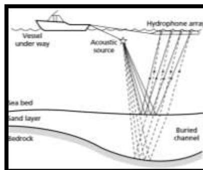
**Figure 3.** Seismic Reflection Survey at Sea [9].
